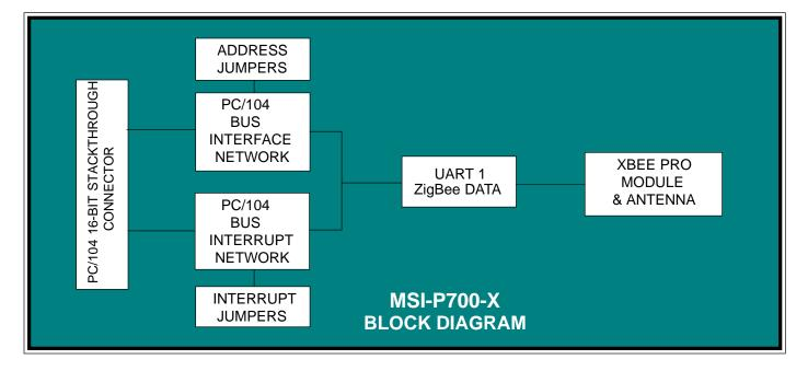
from 1200 to 115,200 bits/s. Automatic hardware RTS and CTS flow control is used to prevent overflow of the local receiver and remote receiver FIFOs. The card I/O address is jumper selectable for COM1 thru COM4 with an optional 16-bit offset address. Interrupts are jumper selectable for IRQ3 thru IRQ5 and IRQ9 thru IRQ15.
